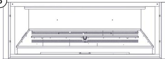
REMOVE ALL MEDIA FROM THE APPLIANCE, VACCUUM ANY REMAINING MEDIA OR DEBRIS FROM THE FIREBOX.
